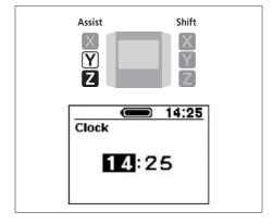
**2.** Pressing the Assist-X enables the set value and moves you to the minutes setting.
