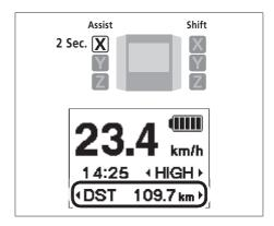
**2.** Release the finger when the DST indication starts blinking.
