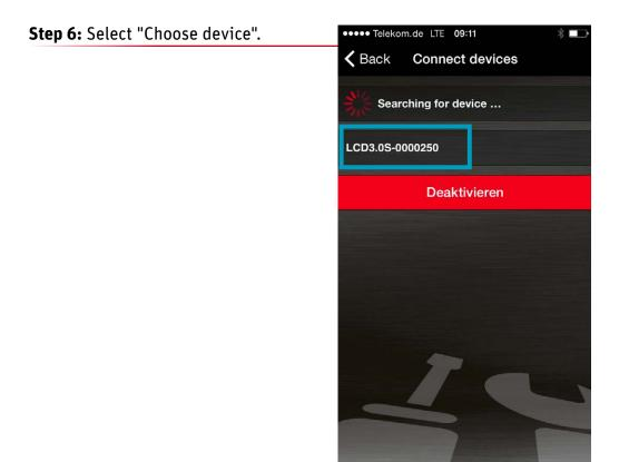
Choose the Impulse Evo bike that you want to connect to your smartphone. You will find the number of your E-Bike on the back of the Impulse Evo Smart Display. This is the 8-digit SN number. The final digits of this number are the ones to need to check.
